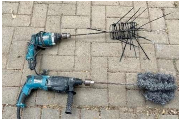
FIGURE 3. Lightweight Brick Mixer
