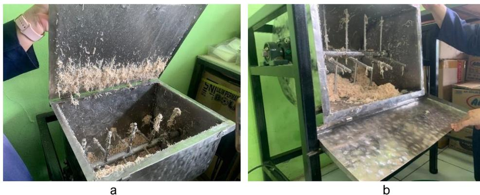
FIGURE 7. (a) Chicken meat has been shredded by machine, (b) Chicken Meat Dispensing Process
