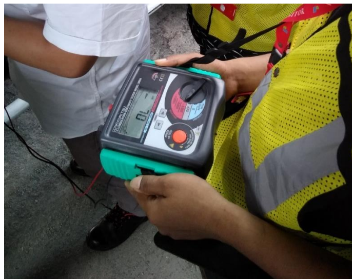
FIGURE 4. Insulation resistance test results using a megger
