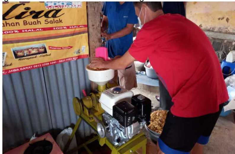
Figure 3. The process of milling dodol with a machine
