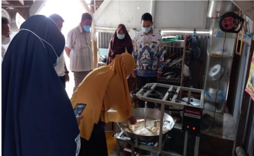
Figure 4. The process of stirring dodol with an automatic stirrer
