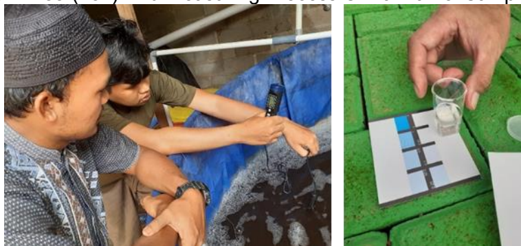
Figure 4. Measuring DO, Nitrit, Nitrat, Posphate Of The Vannamei Shrimp Culture Water
