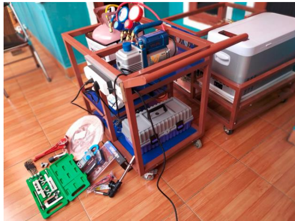
Figure 1. A/C service equipment and accessories
