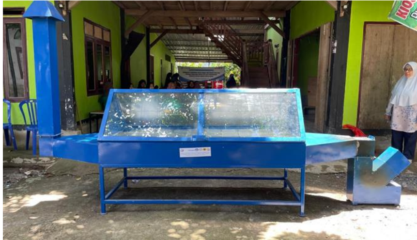
FIGURE 3. The hybrid drying technology utilising a rocket stove
