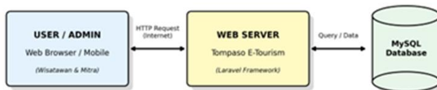
FIGURE 2. The System Architecture Diagram illustrates the data flow between the User Interface, Web Server, and Database
